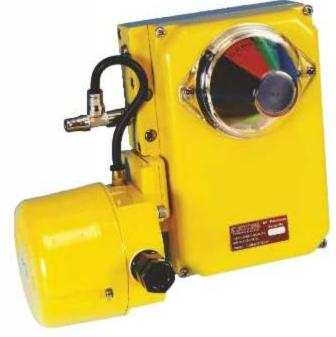
The optional Kinetrol I/P Controller is mounted in place of the standard diaphragm housing on the side of the positioner case. The positioner can still be mounted in any orientation and gives an angular output position which is proportional to the input current control signal between 4-20mA.
